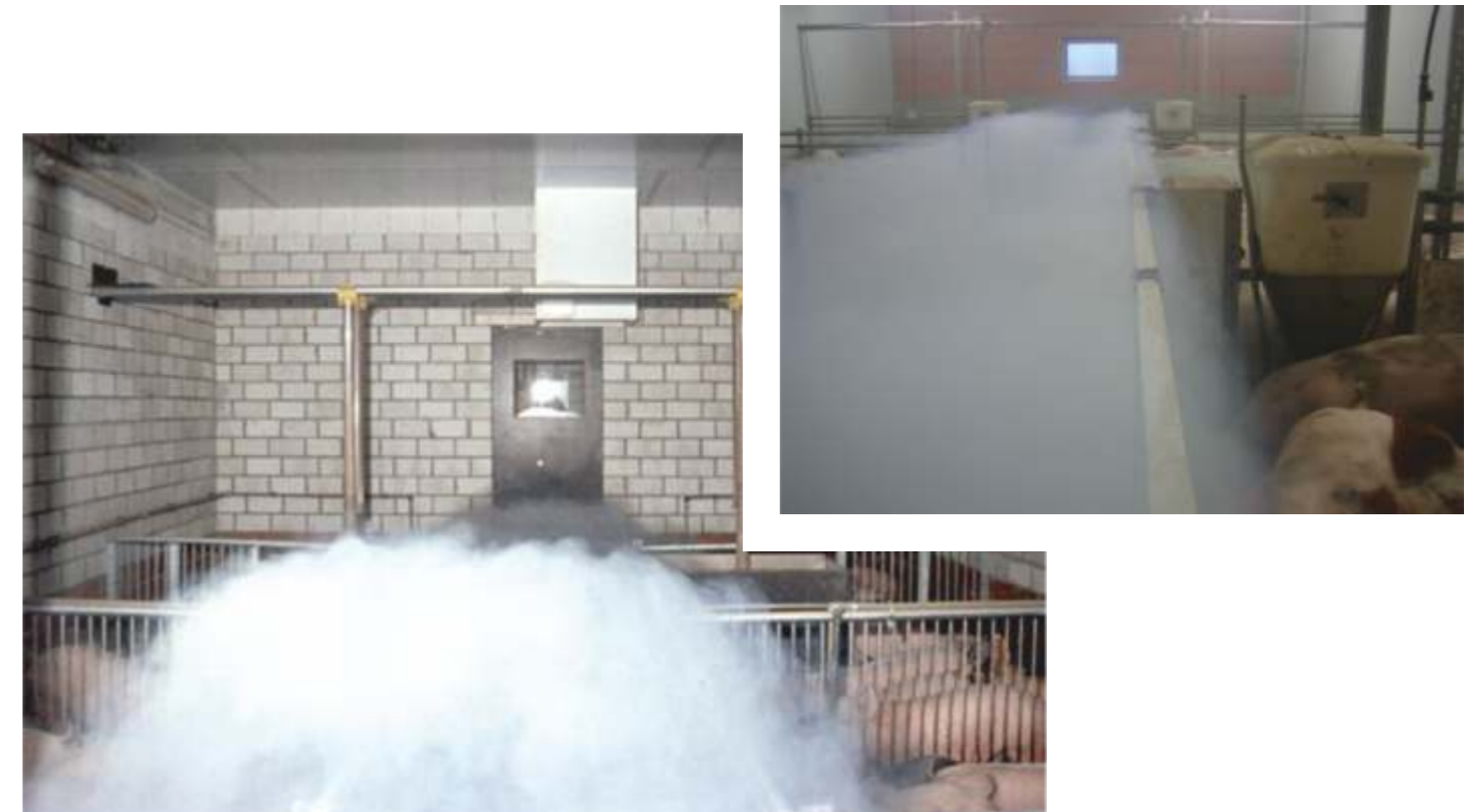
Mist illustration of corridor ventilation system
